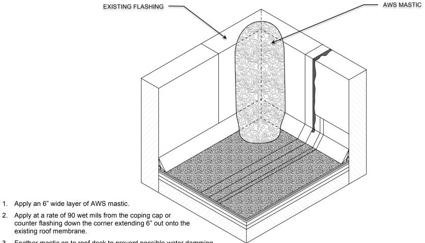
3. Feather mastic on to roof deck to prevent possible water damming.
