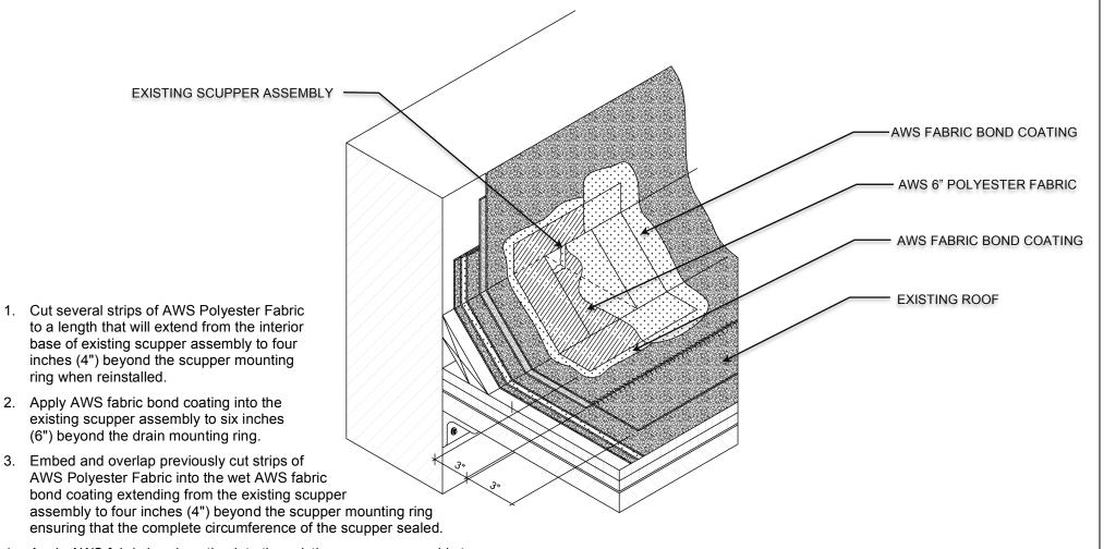
4. Apply AWS fabric bond coating into the existing scupper assembly to six inches (6") beyond the drain mounting ring, completely encapsulating the AWS Polyester Fabric.
