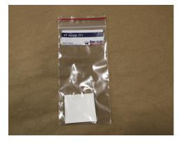
Patch sample of High-Tensile Acrylic 211 roof coating
