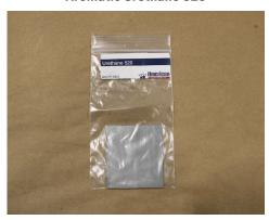
Patch sample of Aromatic Urethane 520 roof coating
