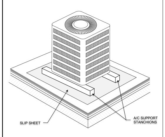
NOTE: Stanchions should be in good condition. Rotten and/or deteriorated stanchions should be replaced. Slip sheet should extend a minimum of 6" beyond the outside edges of stanchion.
