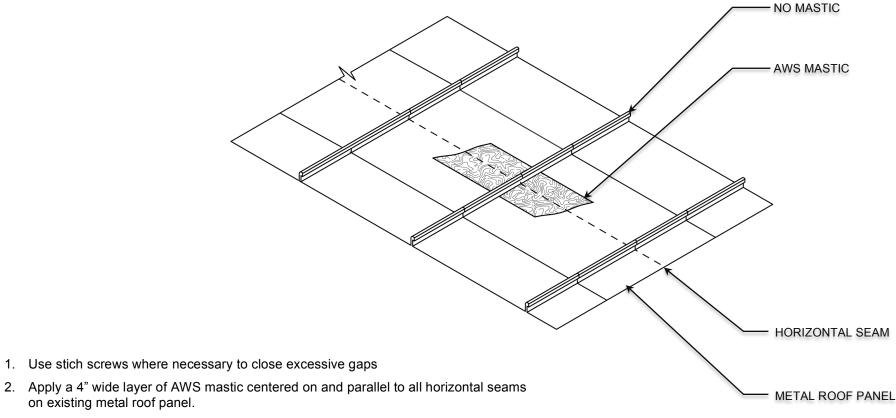
3. Apply AWS mastic at a minimum rate of 60 mils, ensuring all voids in flat area of panel are filled.
