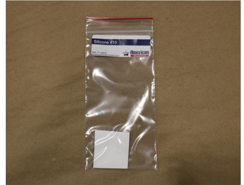
Patch sample of Silicone 410 roof coating
