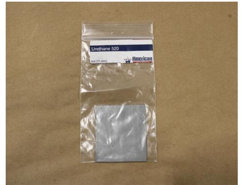
Patch sample of Aromatic Urethane 520 roof coating
