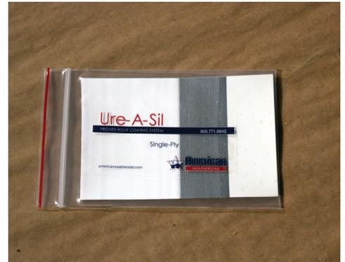
3" x 5" sample comprised of Aromatic Urethane 520 base coat and Silicone 410 top coat applied over granulated modified bitumen
