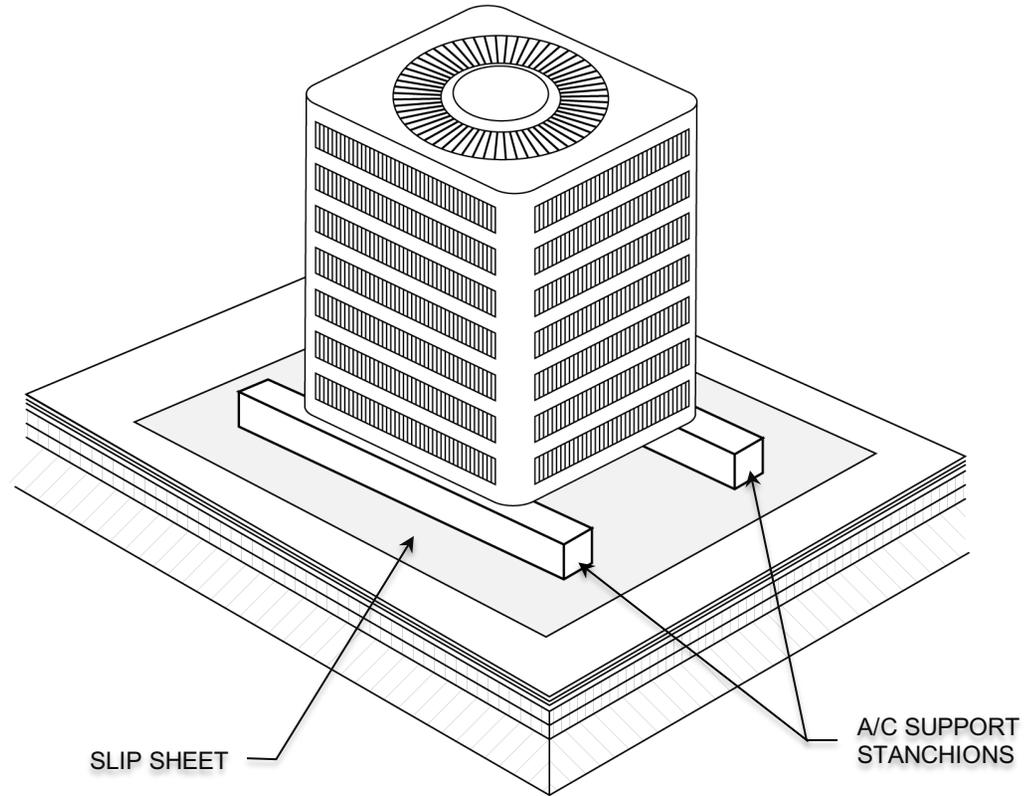
NOTE: Stanchions should be in good condition. Rotten and/or deteriorated stanchions should be replaced. Slip sheet should extend a minimum of 6" beyond the outside edges of stanchion.
